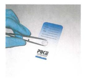
Place the pellet on the 13 mm Magnetic Pellet Holder and secure it with a magnet, or attach it to the adhesive ring of a disposable card. Place in the slide holder of your spectrometer for analysis.
