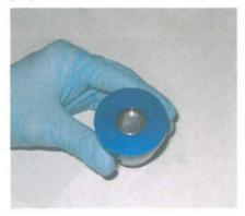
When the bottom anvil emerges sufficiently, remove it gently with your fingers. The pellet, resting on the upper polished anvil, will be exposed at this point. Keep pressing gently at the surface until the second anvil is exposed. If necessary, the ejector ring may be placed underneath to extend the travel of the piston.
