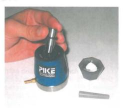
Place piston in the well of the block assembly. The O-ring provides support for the piston and it seals the gap between the piston and the barrel when vacuum is applied.
