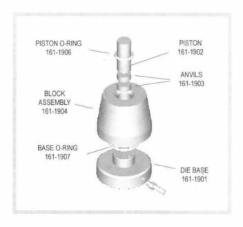
The PIKE Evacuable KBr Die Kit features the following components: a stainless steel base with vacuum outlet, the main die block with a 13-mm cylinder, two anvils, a plunger, and an ejector ring. Components are made of hardened stainless steel, and surfaces that come in contact with the sample are highly polished. Two different size O-rings are used to seal the base/die assembly and the plunger.
